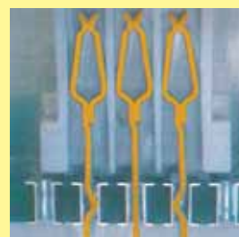
Cross section of a connector with kinked contacts assembled to a pcb
