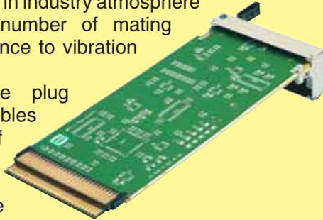
of  $1.6 \text{ mm} \pm 10 \%$ . Thanks to the special design of the mating face, the plug halves the mating forces compared to a PCB. The plug connector fits into the AMC.0 specification when mounted to the PCB and can hence be used in both MicroTCA™ and ATCA® environments.
