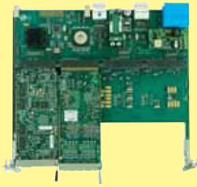
AdvancedTCA<sup>®</sup> carrier board with AdvancedMC<sup>™</sup> modules
