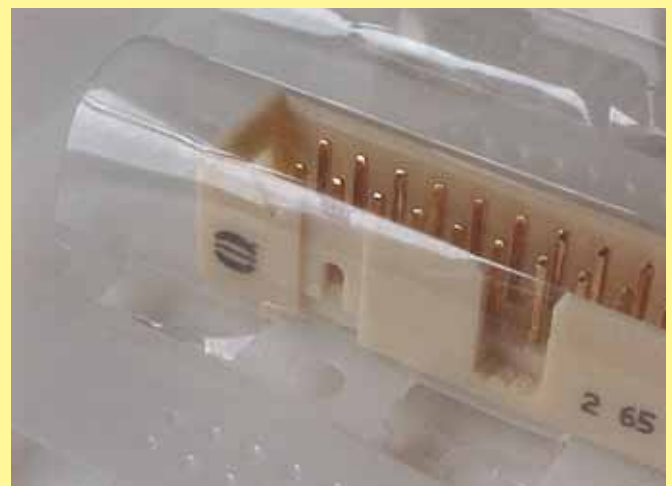
HARTING connector mounted in a tape ready for placement using an odd form assembly station.
