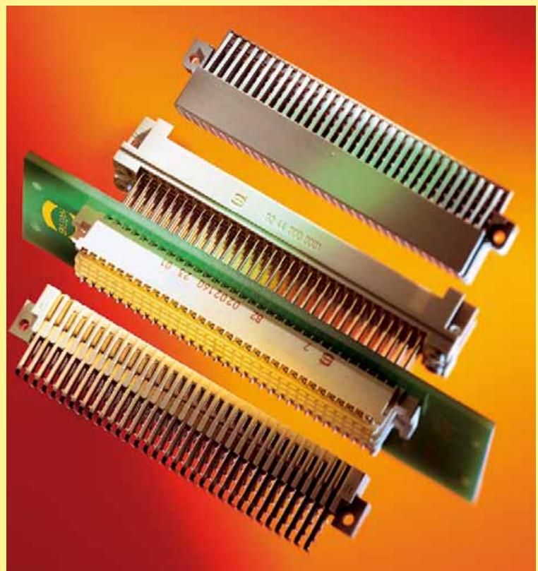
With the increase in processing speeds and data transmission rates, 3 row DIN 41612 connectors have reached their limit, so the VME standard needs to be enhanced further.
