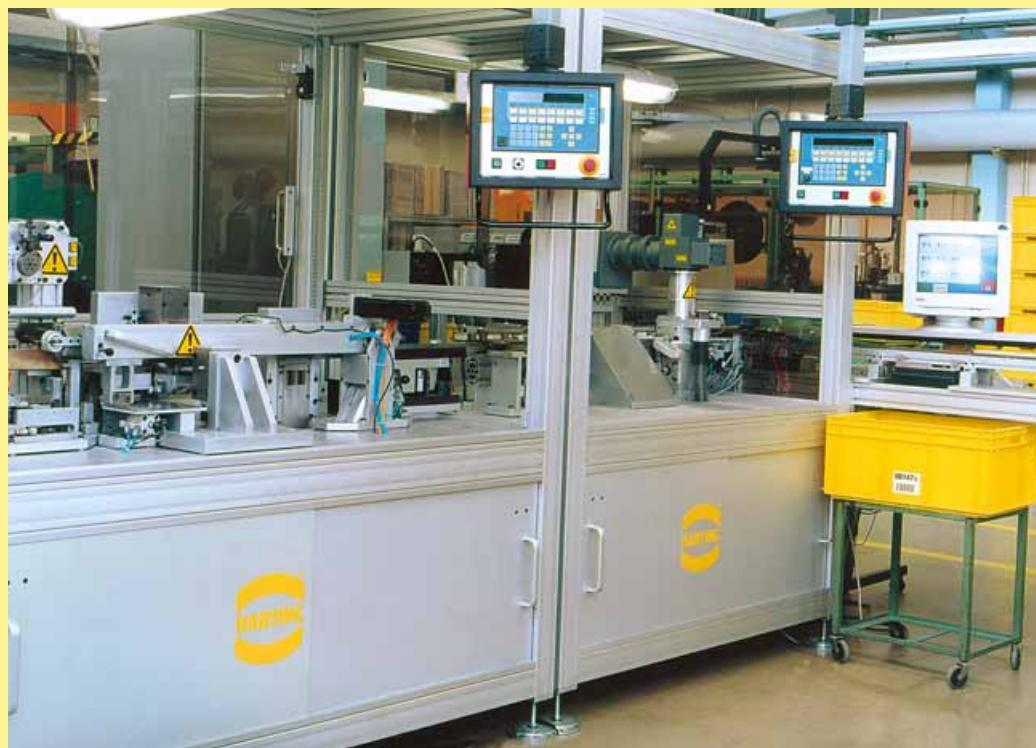
Fully automated assembling and printing devices, monitored through video camera inspection systems and laser technology.
