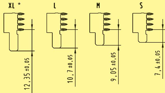
The compact, high temperature moulding can be loaded with up to four high current contacts. Four different contact lengths are available from 7.4 mm to 12.35 mm. This makes sequenced and non-sequenced loadings possible (e.g. with GND and ENA). Any other contact assignments, also partially loaded, are available on request.
