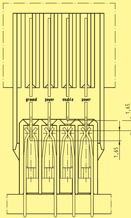
Loaded with four power contacts, each contact can carry up to 20 A @ 70 °C / 80 % derating.
