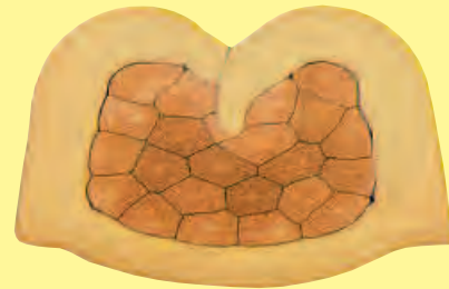
B shape cross section stamped contact
