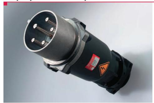
The heavy duty range supplements the plugs and sockets currently covered by EN 60309-2, making available rated currents of 200A, 250A and 400A and rated voltages of up to 1000V. Their design is based on the following standards: IEC 309-1, EN 60309-1,
