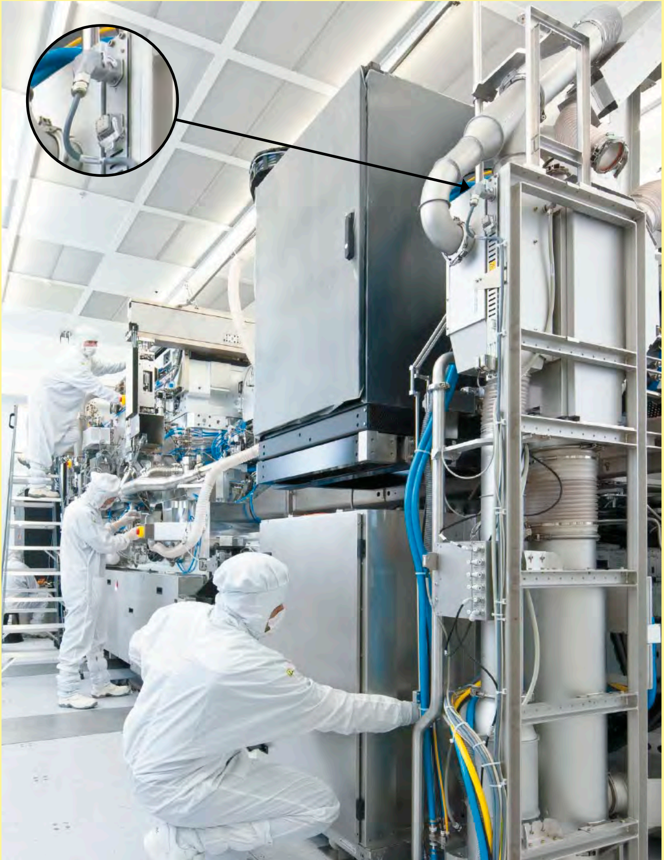
ASML's TWINSKAN NXE platform using Han® Q connectors is the industry's first production platform for extreme ultraviolet lithography (EUVL).
